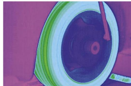
On the tyre testbed: infrared camera detects rolling resistance and heat development of tyre
